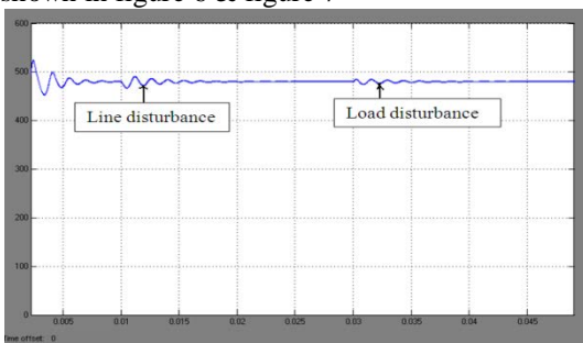
Figure 3 Output voltage waveform for Line & Load disturbance
